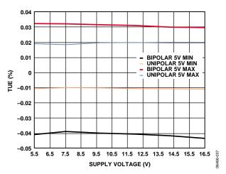
Figure 19. AD5752R Total Unadjusted Error vs. Supply Voltage
