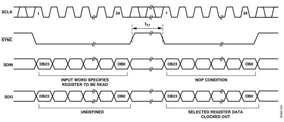
Figure 4. Readback Timing Diagram
