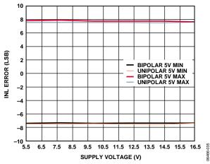
Figure 16. AD5752R Integral Nonlinearity Error vs. Supply Voltage
