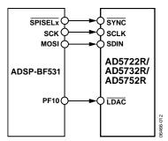
Figure 50. AD5722R/AD5732R/AD5752R-to-Blackfin Interface
