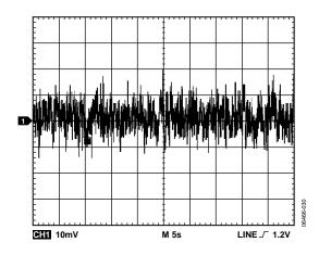
Figure 35. REFOUT Output Noise (0.1 Hz to 10 Hz Bandwidth)
