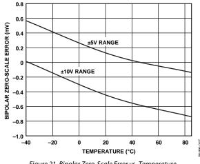
Figure 21. Bipolar Zero-Scale Error vs. Temperature
