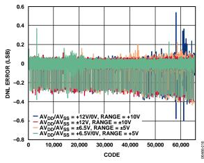
Figure 9. AD5752R Differential Nonlinearity Error vs. Code
