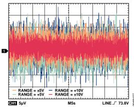
Figure 31. Peak-to-Peak Noise, 100 kHz Bandwidth
