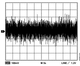
Figure 34. REFOUT Output Noise (100 kHz Bandwidth)
