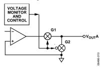
Figure 48. Analog Output Control Circuitry
