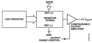
Figure 44. DAC Architecture Block Diagram
