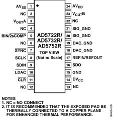
Figure 5. Pin Configuration
