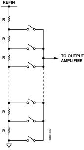
Figure 45. Resistor String Structure
