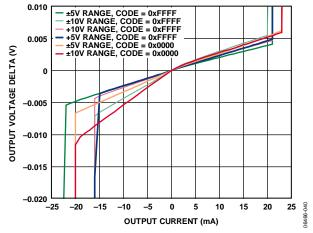
Figure 24. Output Source and Sink Capability
