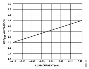
Figure 36. REFOUT Voltage vs. Load Current
