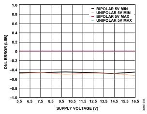
Figure 17. AD5752R Differential Nonlinearity Error vs. Supply Voltage
