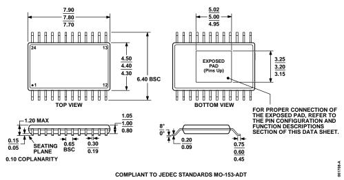
Figure 51. 24-Lead Thin Shrink Small Outline Package, Exposed Pad [TSSOP\_EP] (RE-24) Dimensions shown in millimeters
