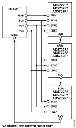
Figure 46. Daisy Chaining the AD5722R/AD5732R/AD5752R
