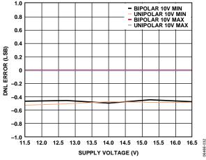
Figure 15. AD5752R Differential Nonlinearity Error vs. Supply Voltage
