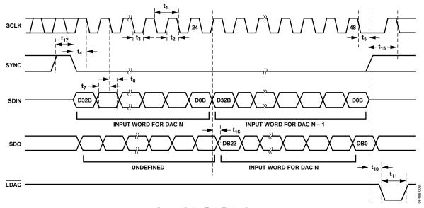
Figure 3. Daisy-Chain Timing Diagram
