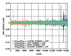
Figure 10. AD5732R Differential Nonlinearity Error vs. Code
