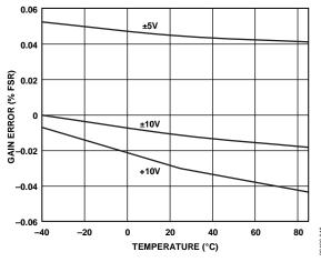
Figure 22. Gain Error vs. Temperature
