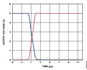
Figure 28. Full-Scale Settling Time, +5 V Range
