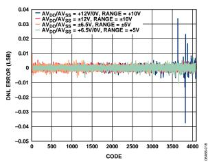
Figure 11. AD5722R Differential Nonlinearity Error vs. Code
