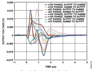
Figure 29. Digital-to-Analog Glitch Energy
