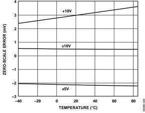
Figure 20. Zero-Scale Error vs. Temperature
