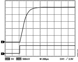
Figure 33. REFOUT Turn-On Transient
