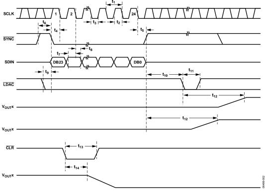
Figure 2. Serial Interface Timing Diagram
